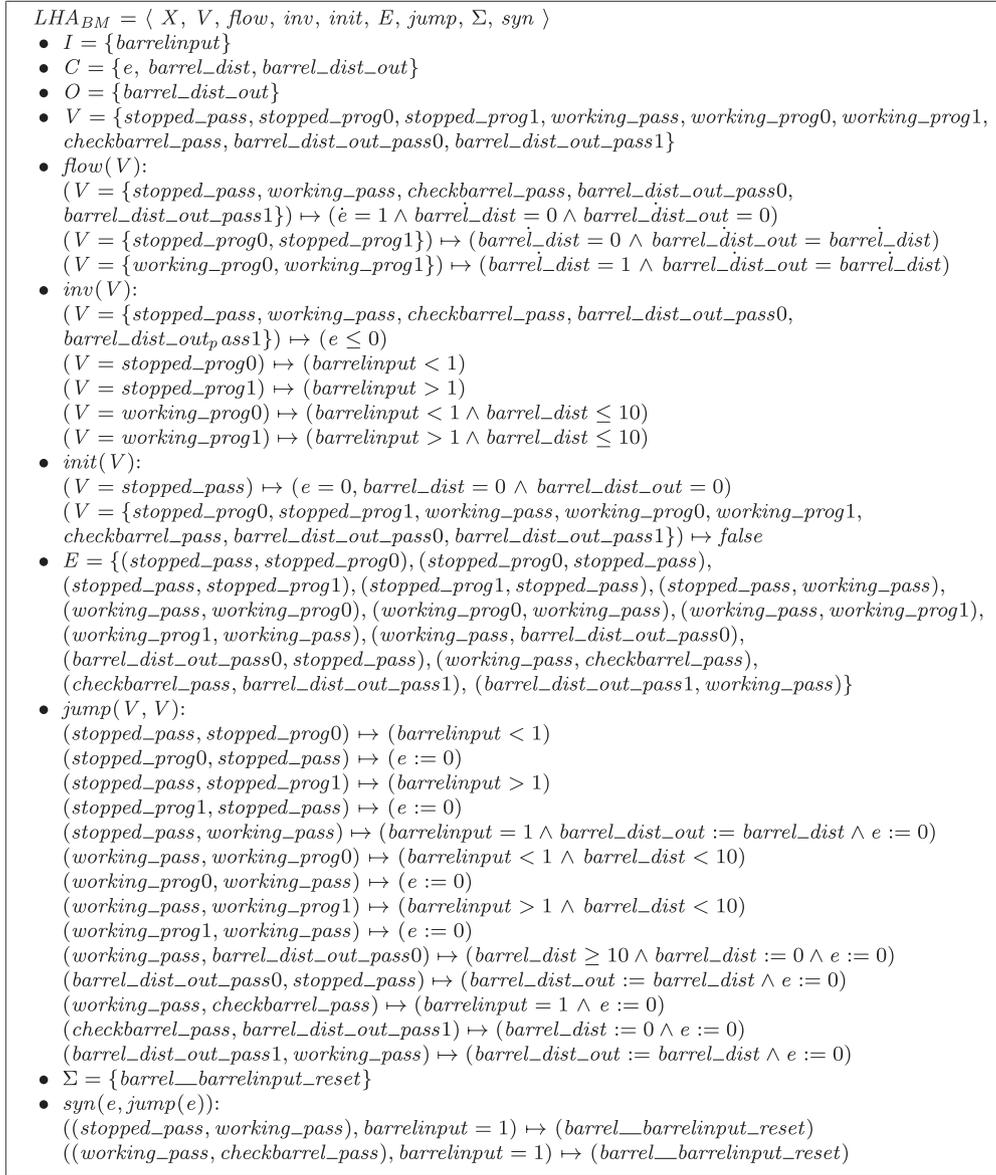
Fig. 30. The formal definition of  $LHA_{BM}$  for the 'Barrel-Mover System'.
