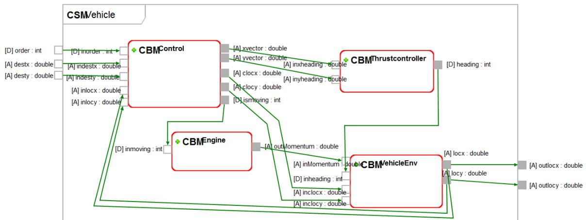
Figure 4 An ECML SM for simplified 'vehicle control system'
