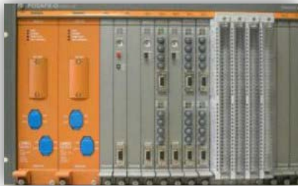
PLC (Programmable Logic Controller)
