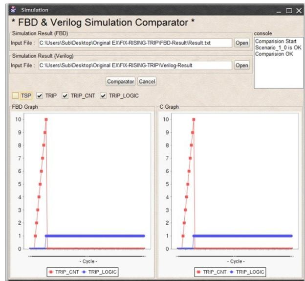
Figure 12 A screen dump of ‘FBD & Verilog Comparator’
