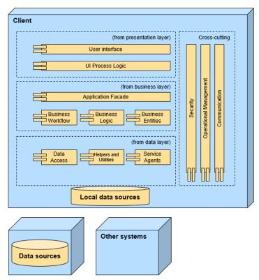
Figure 5. Rich client application reference architecture
