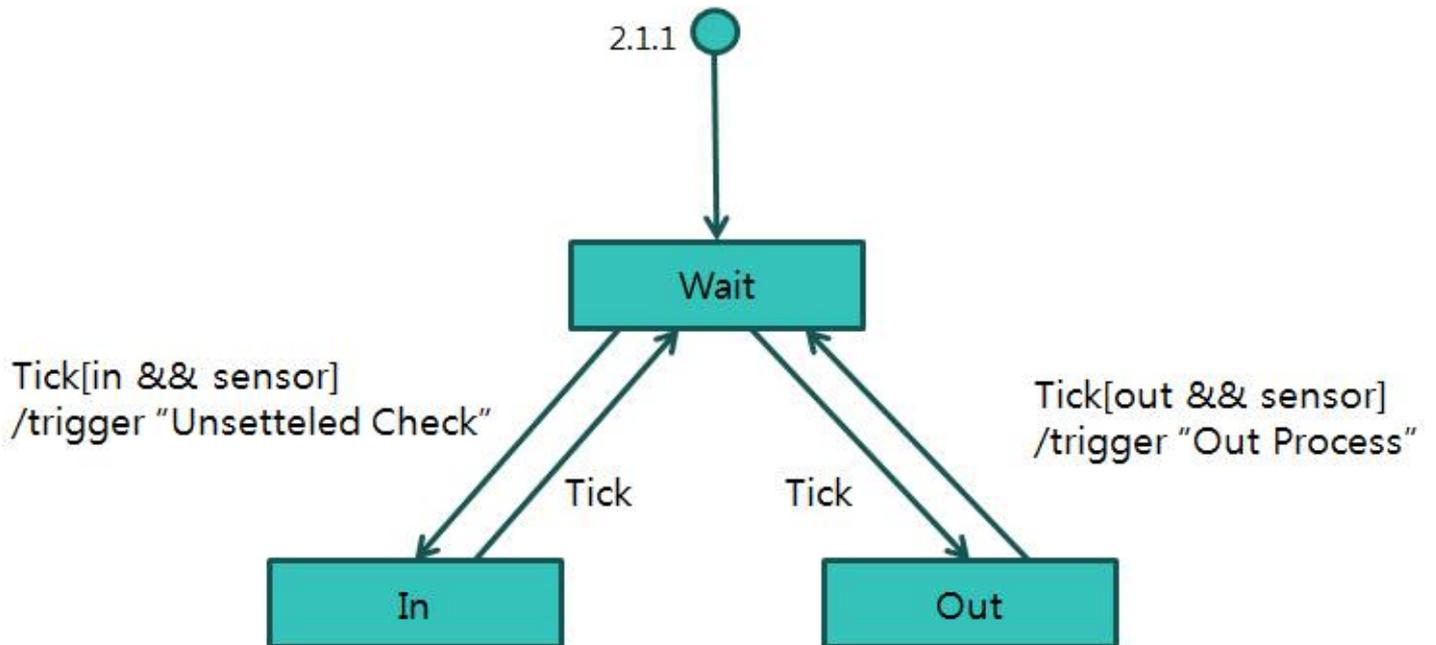
3.2.4.5 State Transition Diagram for Calculated Data Controller2.2.1
